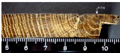
Fig.10. Oak plank, detail: pith.
